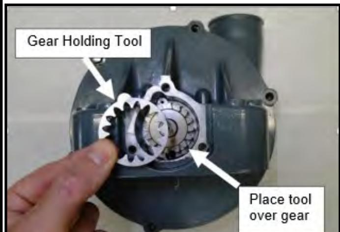
Apply a **small** amount of heat to supercharger impeller nut. Using a 1/4" ratchet and 6-point, 12mm socket loosen nut securing supercharger impeller to shaft by **ROTATING CLOCKWISE**. **NOTE: Threads are left-handed.** If nut is not easily loosened apply a **small** amount of heat and repeat.
