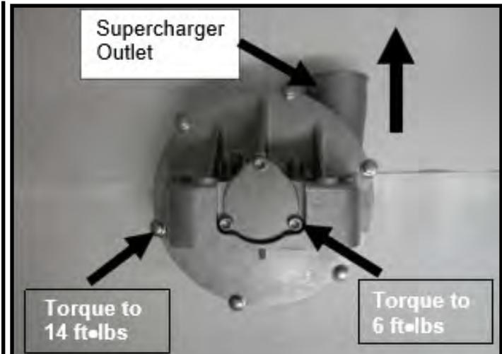
On top of supercharger gear housing remove the small bolt and gasket (washer). While rotating supercharger impeller add Yamalube 4M engine oil to pre-lubricate impeller shaft.
