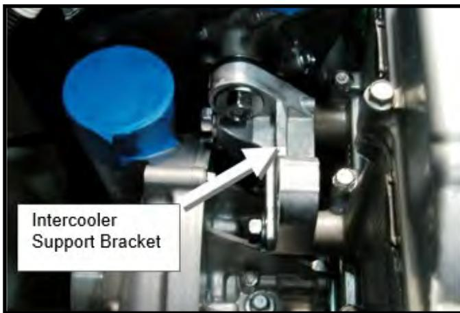
Remove the M8 bolts (4), and M6 bolts (2) from supercharger unit. Remove supercharger unit from engine.
