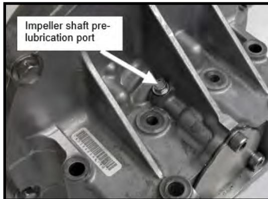
Inspect gasket (washer). If deformed or severely crushed replace with new gasket (washer). Order part# 6S5-14199-00-00. Install bolt and gasket (washer).
