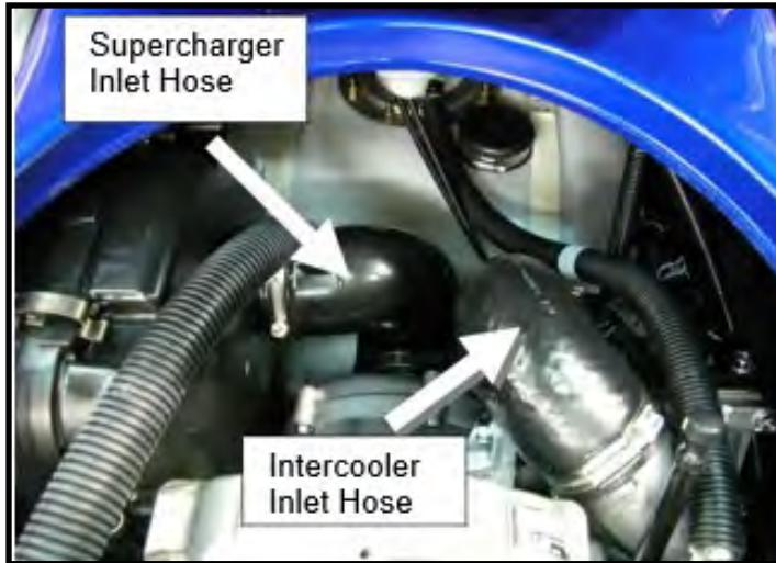
Cover supercharger air outlet and intercooler air inlet with masking tape to prevent debris from entering.
